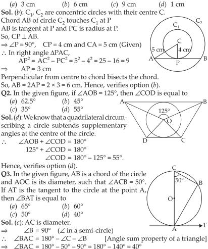
Tangent AT at A and radius OA at A arc at 90°.
