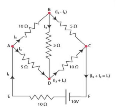
Let I  $_{\mbox{\tiny 1}}$  be the current flowing through the outer circuit
