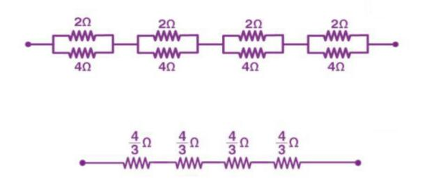
All the four resistors are connected in series. Hence the equivalent resistance R each are (4/3) x 4 = 16/3  $\Omega$
