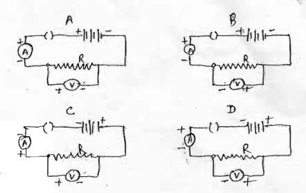
Out of the four circuits shown for studying the dependence of the current on the potential difference across a resistor, the correct circuit is:
