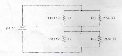
In the figure R1 = 100  $\Omega$ , R2 = 250  $\Omega$ , R3 = 350  $\Omega$  and R4 = 200  $\Omega$  and a battery is connected to the arrangement. Calculate
