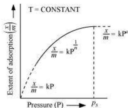
The plot between the extent of adsorption  $\left(\frac{x}{m}\right)$  against the pressure of gas ( $P$ ) at constant temperature ( $T$ ) is called the adsorption isotherm.
