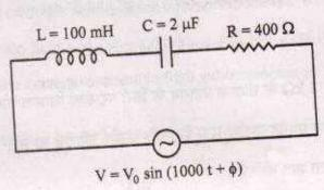
Find the value of the phase difference between the current and the voltage in the series LCR circuit shown below. Which one leads in phase : current or voltage ? (i)
