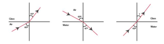
The figures above show the refraction of a ray in air incident at 60° with the normal to a glass-air and water-air interface, respectively. Predict the angle of refraction in glass when the angle of incidence in water is 45° with the normal to a water-glass interface.
